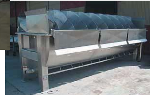
SCT-6 W 1.6 Disinfecting tank
