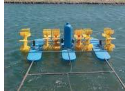
Six impellers aerator
