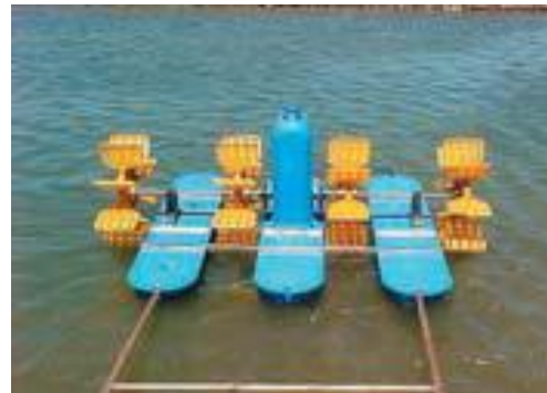
Four impellers aerator
